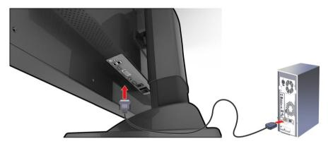
2. Connect the power cord to the power input interface on the display.
