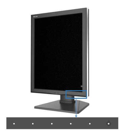
The keys except power key are silkscreen keys. Touch any key except power key to bring up the navigation key icons, as shown below.
